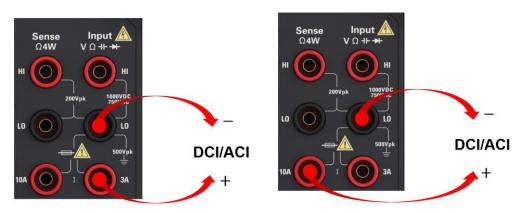
Note: To avoid damaging the multimeter, be sure to follow the instructions below for DC/AC current measurements.
