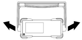
Fig. 1-1 Adjusting the handle
