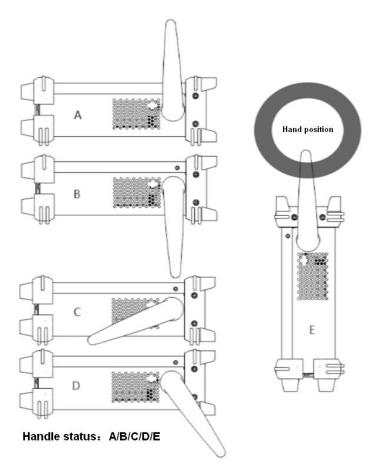
Fig. 1-2 Placing the instrument
